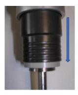
And adaptor AC265-BAYONET is provided with your device. It allow using of bayonet coupling spindle as MS RV/LV, MS KREBS, MS VANE or MS BV. To use it, you have to remove a littl bit screw on this adaptor, insert bayonet side of spindle inside hole and lock it with provided tool. Please do not insert it too much and check that only conical part of bayonet spindle shaft is visible.
