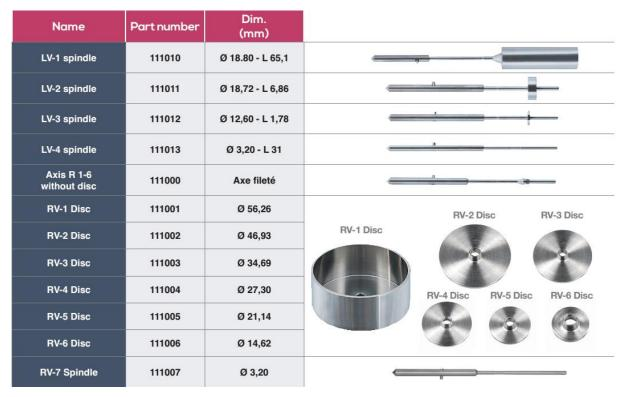
These spindles are composed of two groups. The mobiles L are intended for low viscosity fluids and R mobiles for medium to high viscosities (see tables below with viscosity range in mPa.s):
