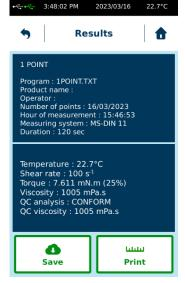
Additionally, to explication on section 2.3.1, you see type of method with name of program on first part of display. On second part of display, you show information about QC analysis if your program had it (see section 2.8.1.1). "QC viscosity" is the measured value used for "QC analysis".
