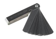
Then you are using a plate-plate measuring system, you have to set in same way the contact position as explained previously. But contact position need to be done by inserting metallic spacer (optional item 100047 as shown on picture above) between MS-PP and 70mm bottom plate. Choice of spacer need to be done according to gap you would like to use with MS-PP measuring system for measurement.
