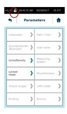
To disable "Locked mode", you must return to service and "Locked mode" and click on "Disable" by entering the 4-digit code.
