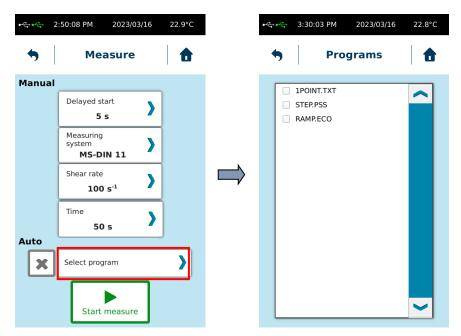
The extension shown next to the program name indicates the type of method according to: "\*.TXT" for 1-point method, "\*.PSS" for step method and "\*.
