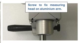
**SECOND STEP:** Insert screw and fix head.
